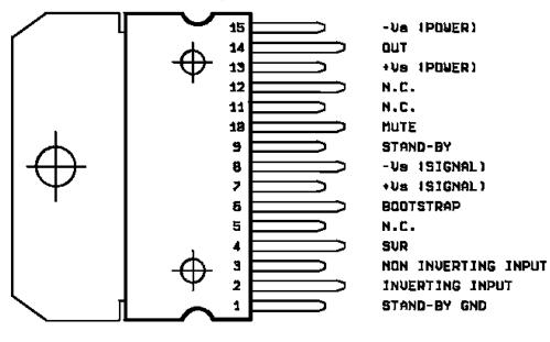
Figure 2. Pin connection
