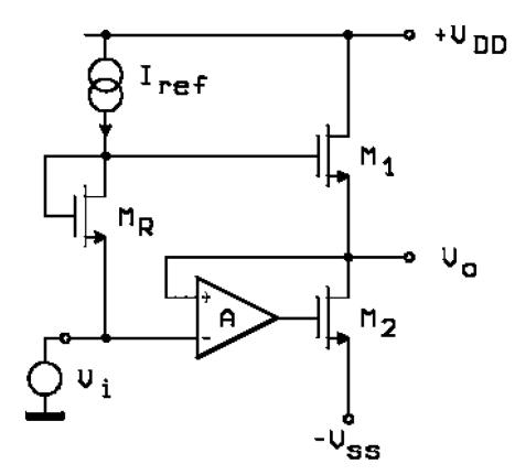
Figure 16. Principle schematic of a DMOS unity-gain buffer
