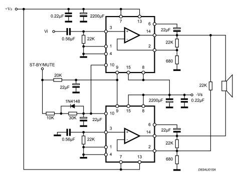
Figure 19. Bridge application circuit
