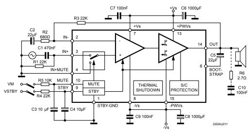
Note: The Boucherot cell R6, C10, normally not necessary for a stable operation it could be needed in presence of particular load impedances at Vs <±25V.
