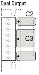
Input Fuse is recommended. Recommended fuse rating = double maximum input current, time delay type. Input Capacitor, C1, is required to meet EN61000 Surge and Fast Transient, otherwise it is not required for normal operation. Output Capacitors C2/C3 are recommended, but not required for normal operation. Typical capacitor values are 1µF MLCC To ensure optimum thermal performance, use large areas of copper on the PCB to assist with heat dissipation and mount the converter vertically.
