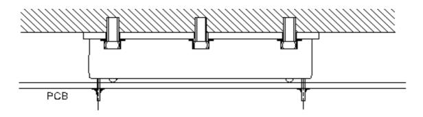
Baseplate Case Fixing - Anti Vibration Mounting onto PCB
