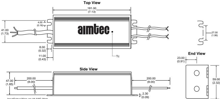
Input/Output Wires are 18 AWG 20cm
