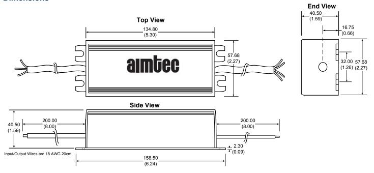
NOTE: to adjust the output current connect a 20K Ohm pot between blue and white wire
