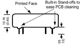
All dimensions are typical: millimeters (inches) Pin Diameter:  $0.50 \pm 0.05 (0.02 \pm 0.002)$ Pin Pitch Tolerance:  $\pm 0.35 (\pm 0.014)$ Case Tolerence:  $\pm 0.5 (\pm 0.02)$
