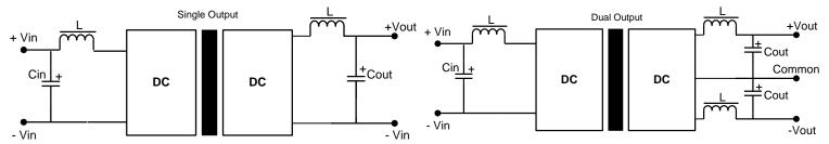
If it is required to decrease the input/output ripple an "LC" filter network can be installed on the input and output of the converter (see above).
