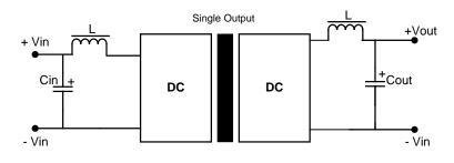
If it is required to decrease the input/output ripple an "LC" filter network can be installed on the input and output of the converter (see above).
