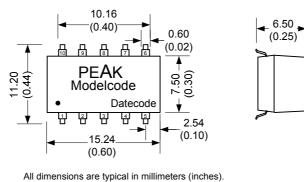
All dimensions are typical in millimeters (inches). - Pin pitch tolerance: +/-0.35 (+/-0.014) - Case tolerance +/-0.5 (+/-0.02) Specification may change without notice.
