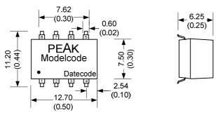
All dimensions are typical in millimeters (inches).
