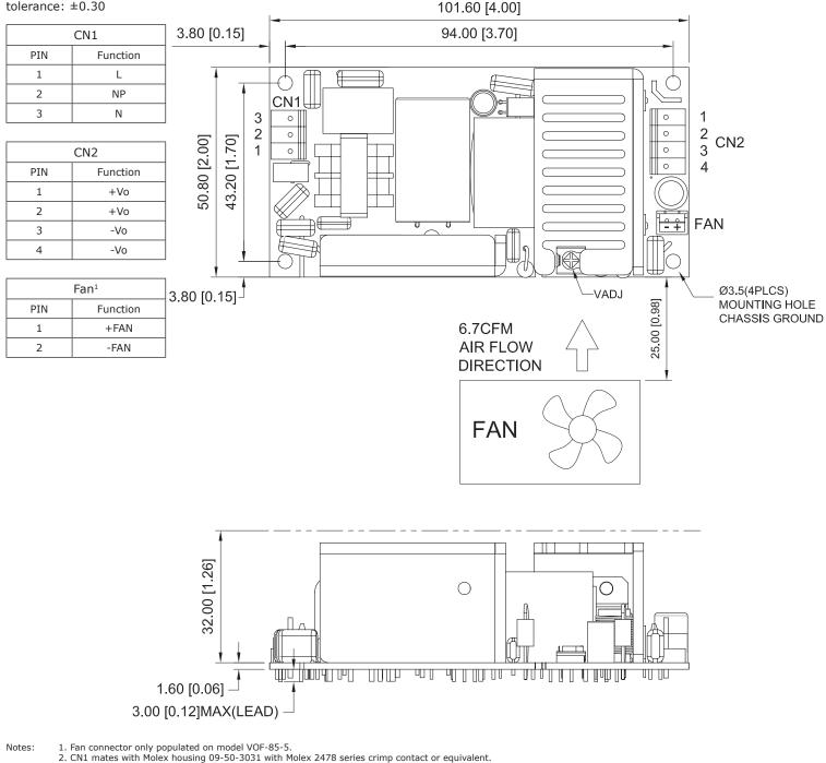
CN2 mates with Molex housing 09-50-3041 with Molex 2478 series crimp contact or equivalent.
