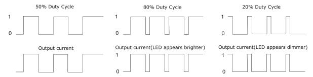
For the rated frequency PWM dimming, the output current of driver matters to the pulse width of the PWM signal, and the numerate please refer to the following formula:
