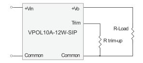
Figure 15. Trim-up Voltage Setup The value of Rtrim-up defined as:
