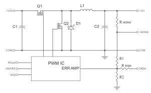
Figure 1. Electrical Block Diagram
