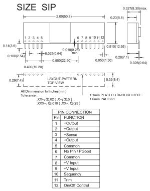
Figure 17 VPOL10A-12W-SIP Mechanical Outline Diagram
