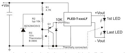
The selection of components for the thermal feedback circuit is not only dependent on the choice of R2 and R3, but also on the amount of heat sink area required to extract heat from the LEDs. To maximize the light output at high ambient or operating temperature conditions, the LEDs must have a sufficient thermal
