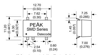
All dimensions are typical in millimeters (inches).
