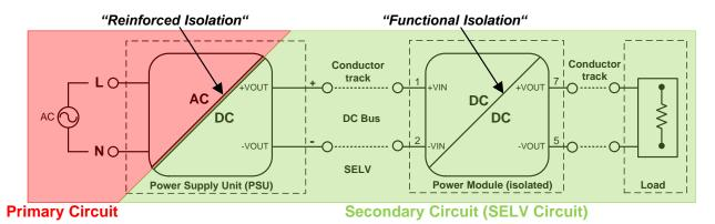
The 1779205x4 Magl<sup>3</sup>C Power Modules are only intended to be used as a CLASS III equipment according to the UL60950-1 standard. That requires that the Power Module is supplied by a **SELV** (safe extra low voltage) circuit which provides protection against electric shock. There are no HAZARDOUS voltages present in CLASS III Equipment.
