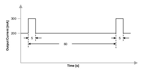
**Note:** The overload current of 300mA can be supplied for maximum 5s and requires a 55s recovery time till next overload event.
