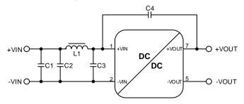
Component Values for Class B filters for the EN55022: C3 is an optional MLCC cap to build up a PI - Filter
