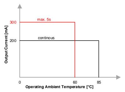
Note: Valid for 5 LFM = 0.03m/s natural convection cooling / horizontal orientate
