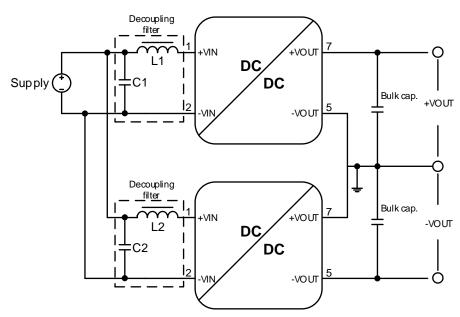
**Note:** A decoupling filter is present to avoid oscillations between the two Power Modules. The decoupling filter doesn't replace the EMI input filter.
