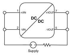
Connect all input – and output terminals together (see Figure) before connecting the supply voltage. When testing, set the cut-off current to 1mA.
