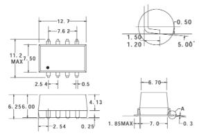
All dimensions in mm. All pins on a 2.54 mm pitch. Tolerance:  $\pm 0.25$ mm
