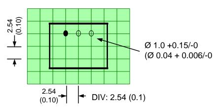
Dimensions are typical values: mm (inch) General Tolerance: ± 0.25 (± 0.01) Pin Tolerance: ± 0.1 (± 0.004)
